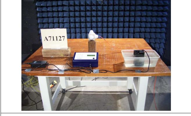
Figure B1. Radiated RF Immunity Test Setup – Front Side.
