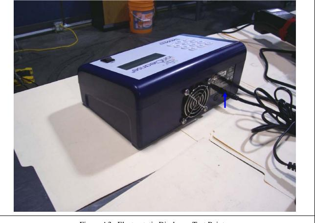
Figure A3. Electrostatic Discharge Test Points.
