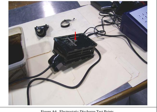
Figure A6. Electrostatic Discharge Test Points.
