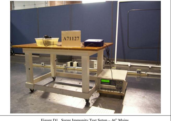
Figure D1. Surge Immunity Test Setup – AC Mains.
