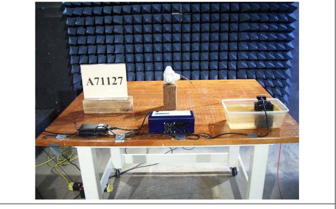
Figure B3. Radiated RF Immunity Test Setup – Back Side.
