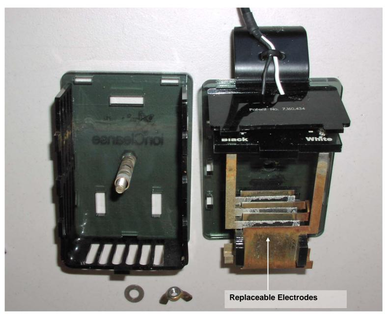
Figure 11: Exposed Interior View of the Array
