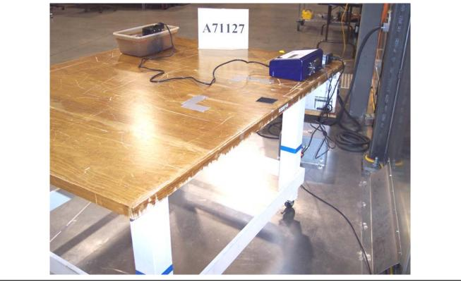
Figure C5: Conducted Emissions Test Setup - Back
