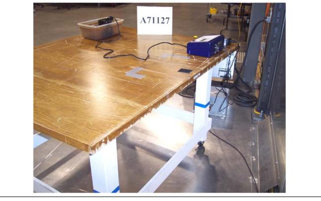
Figure B5: Conducted Emissions Test Setup - Back
