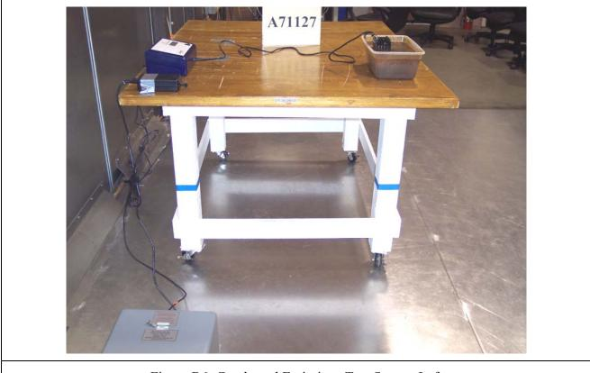
Figure B6: Conducted Emissions Test Setup - Left
