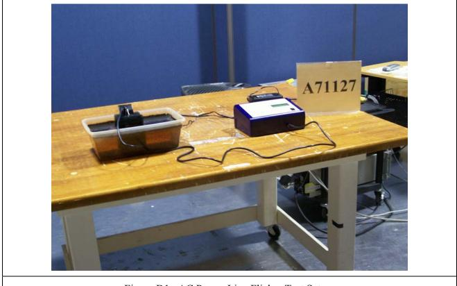
Figure D1. AC Power Line Flicker Test Setup.
