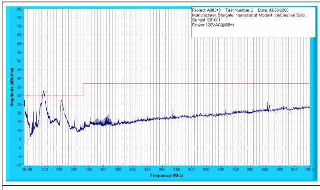
Figure A1: Radiated Emissions Prescan – 30MHz – 1GHz
