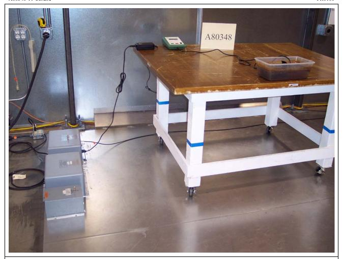
Figure C3: Conducted Emissions Test Setup - Front
