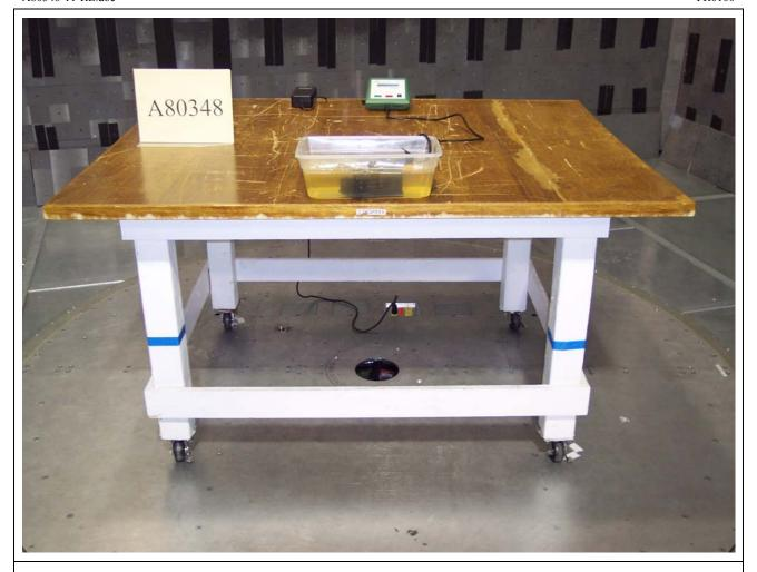
Figure A2: Radiated Emissions Test Setup - Front
