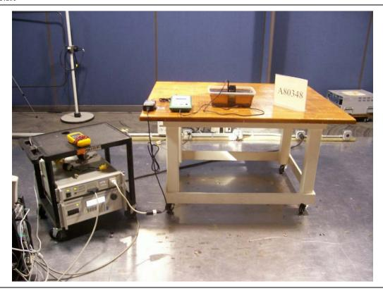
Figure D1. AC Power Line Flicker Test Setup.
