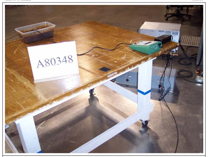
Figure C6: Conducted Emissions Test Setup - Back
