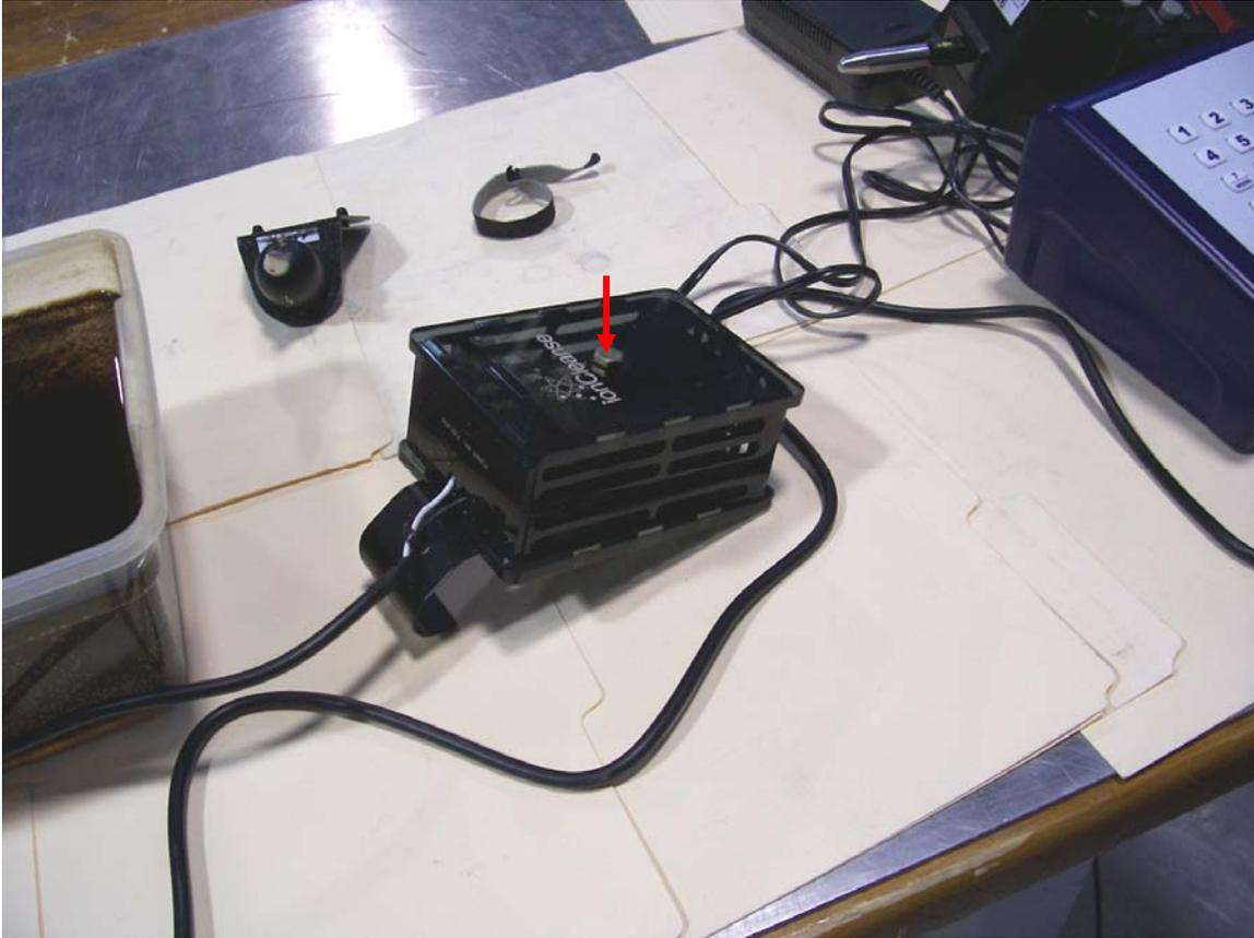
Figure A6. Electrostatic Discharge Test Points.
