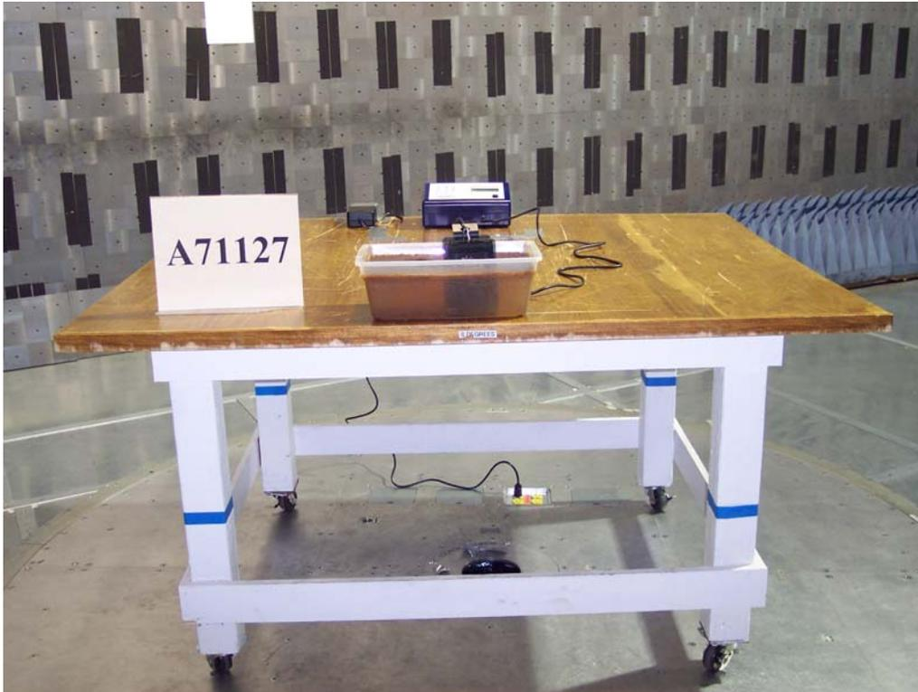
Figure A2: Radiated Emissions Setup - Front
