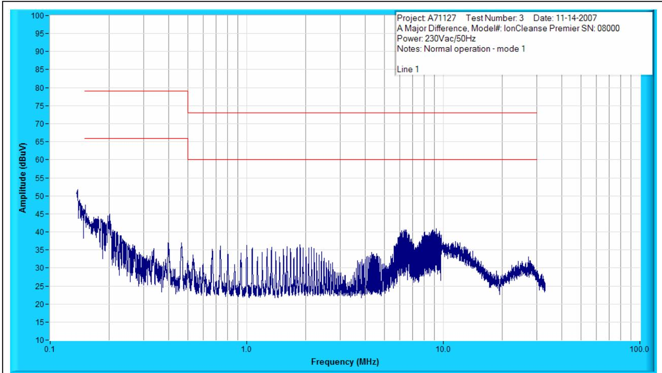
Figure B1: Conducted Emissions Prescan - Line 1.
