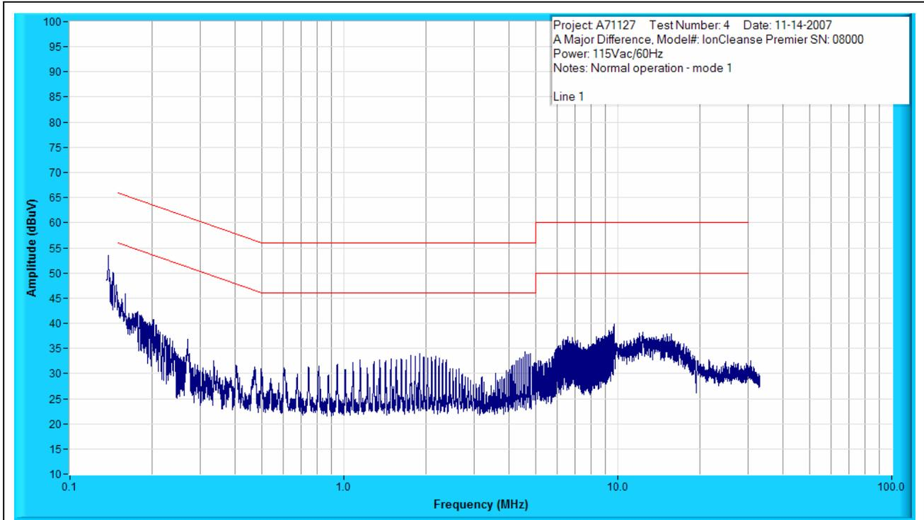
Figure C1: Conducted Emissions Prescan - Line 1.
