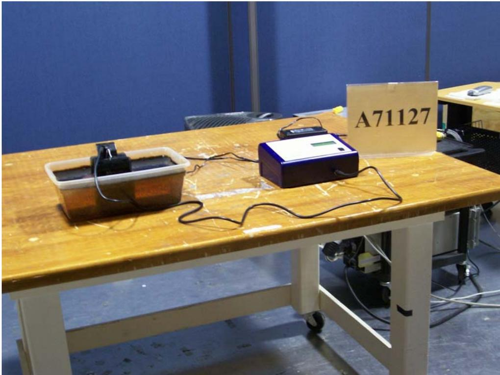
Figure D1. AC Power Line Flicker Test Setup.
