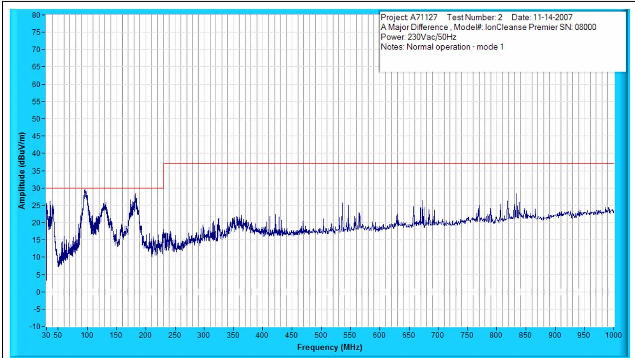
Figure A1: Radiated Emissions Prescan – 30-1000 MHz.
