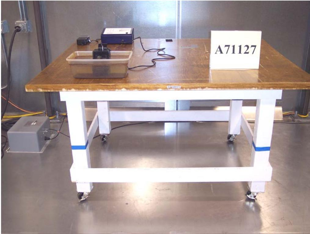
Figure B3: Conducted Emissions Test Setup - Front
