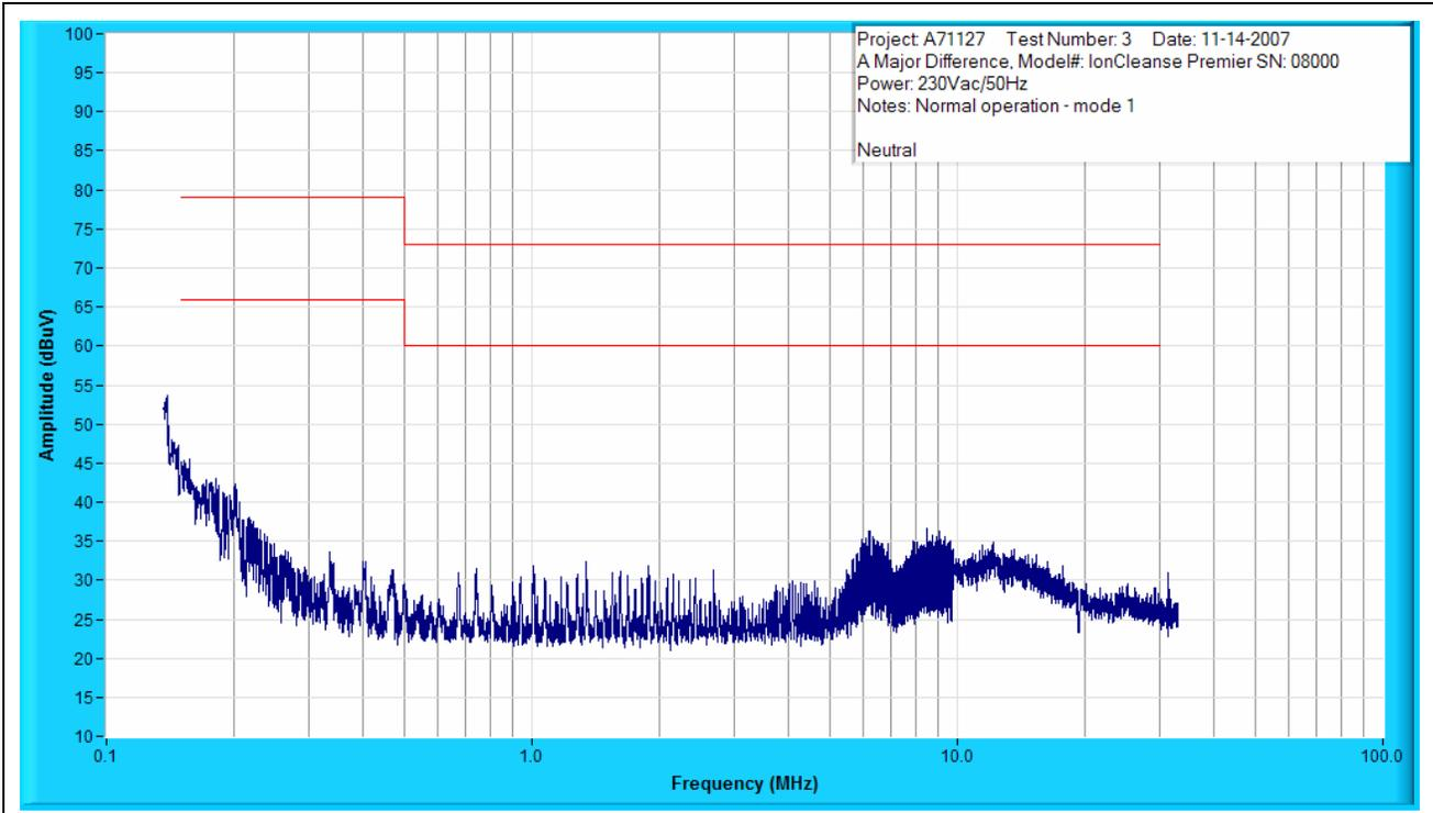
Figure B2: Conducted Emissions Prescan - Neutral.
