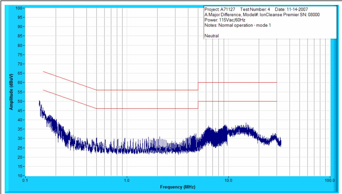
Figure C2: Conducted Emissions Prescan - Neutral.
