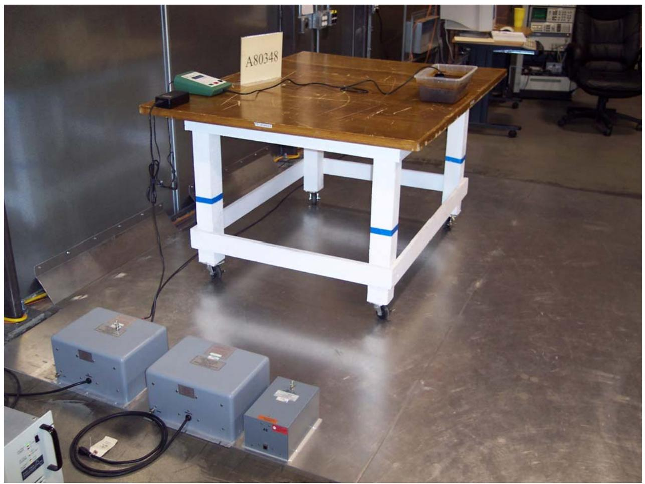
Figure B4: Conducted Emissions Test Setup - Left
