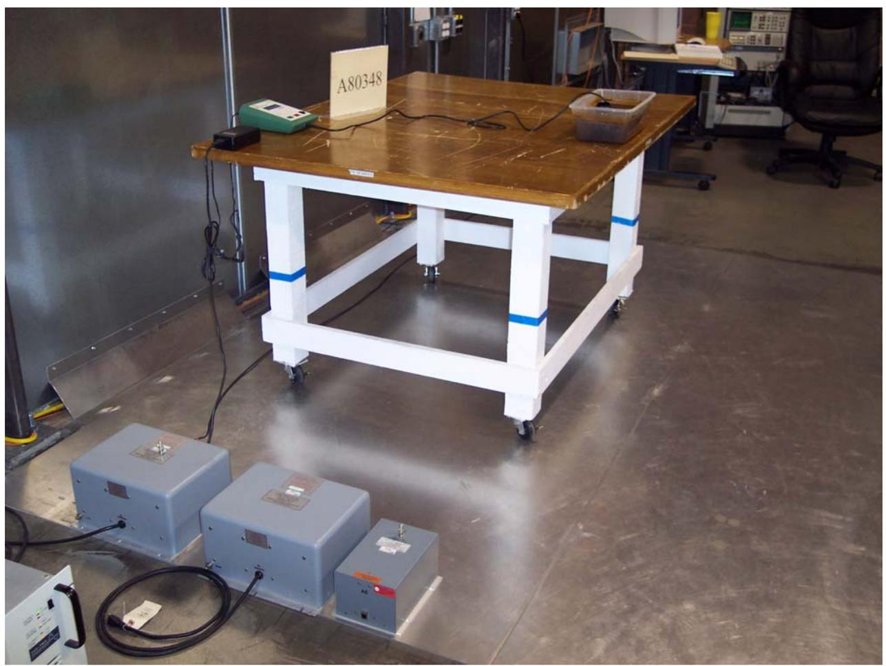
Figure C4: Conducted Emissions Test Setup - Left
