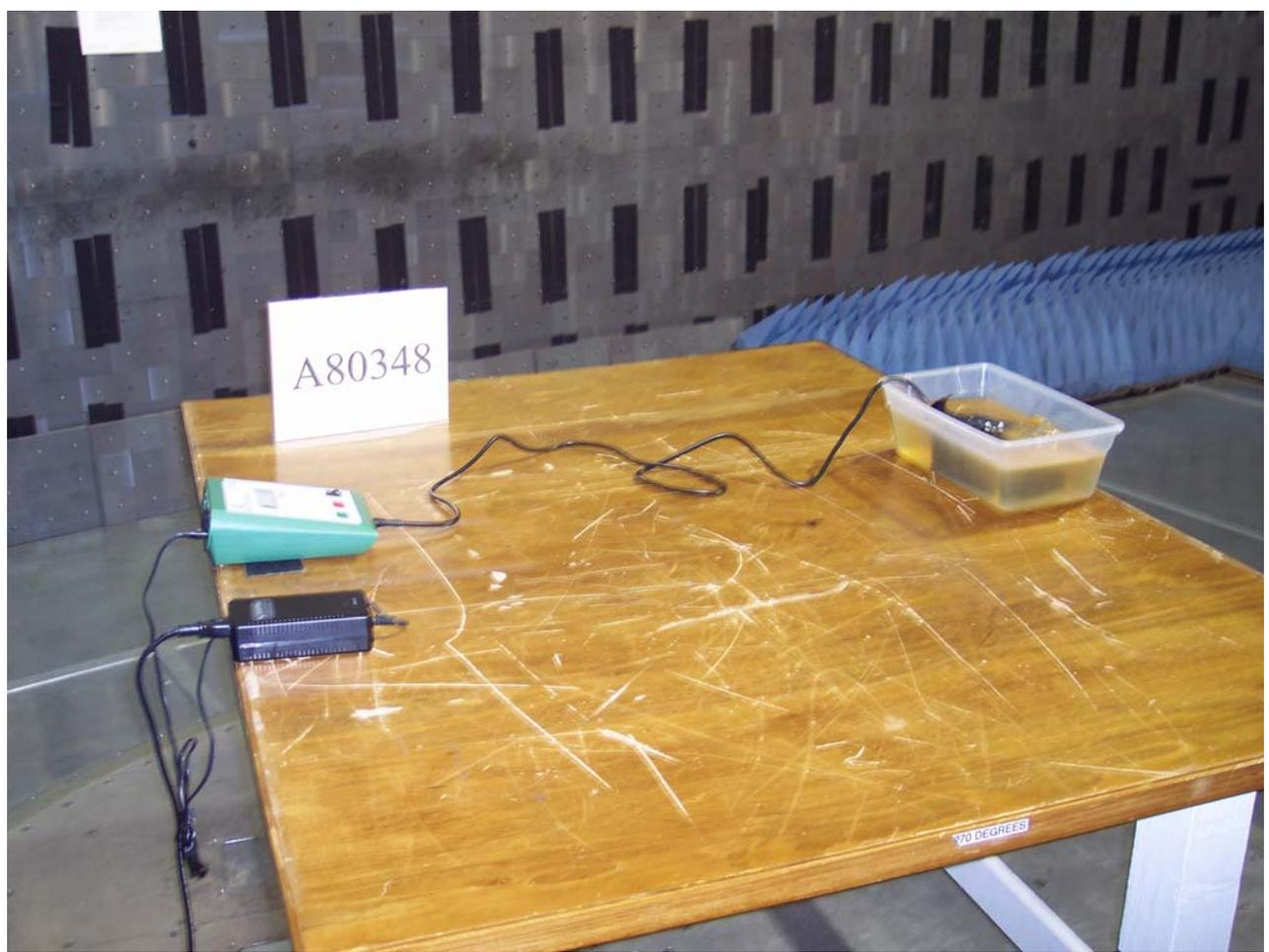
Figure A5: Radiated Emissions Test Setup - Left
