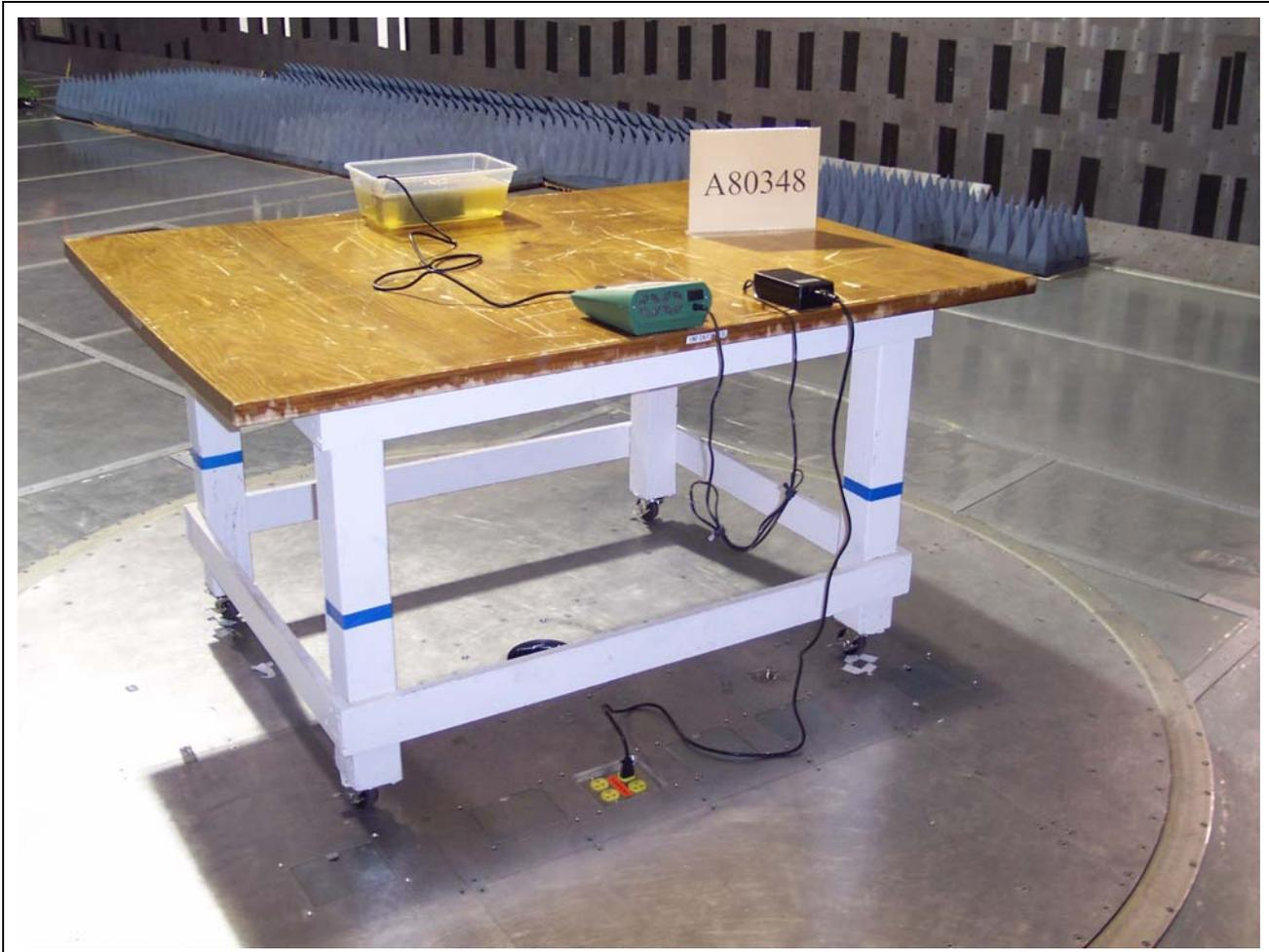
Figure A4: Radiated Emissions Test Setup - Back
